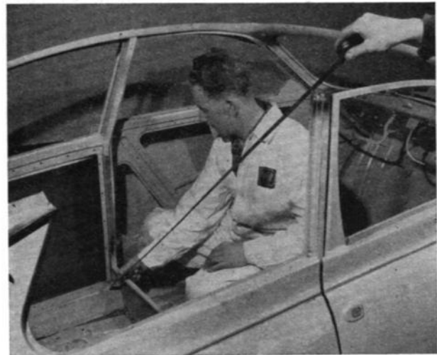
DIAGONAL MEASUREMENT OF CENTER PILLAR
