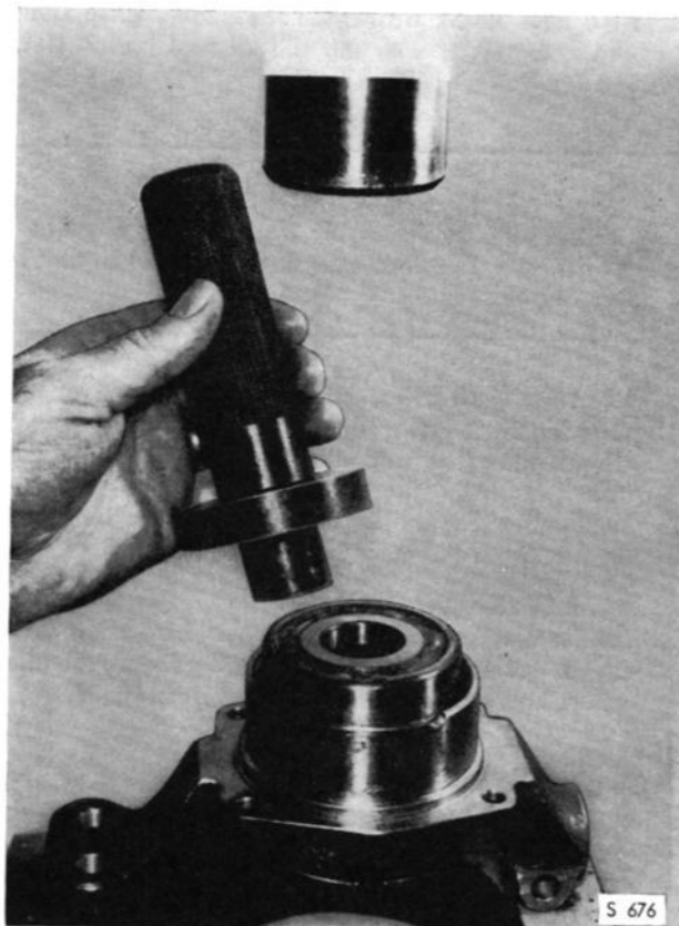
PRESSING IN THE BALL BEARING IN THE STEERING KNUCKLE, TOOLS 784030 AND 784075. THE MARK ON THE BALL BEARING FACING OUTWARDS
