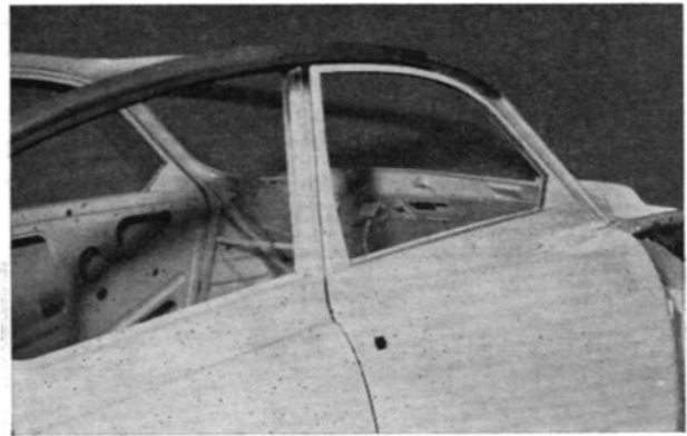
FITTING NEW ROOF RAIL AND MOULDING
