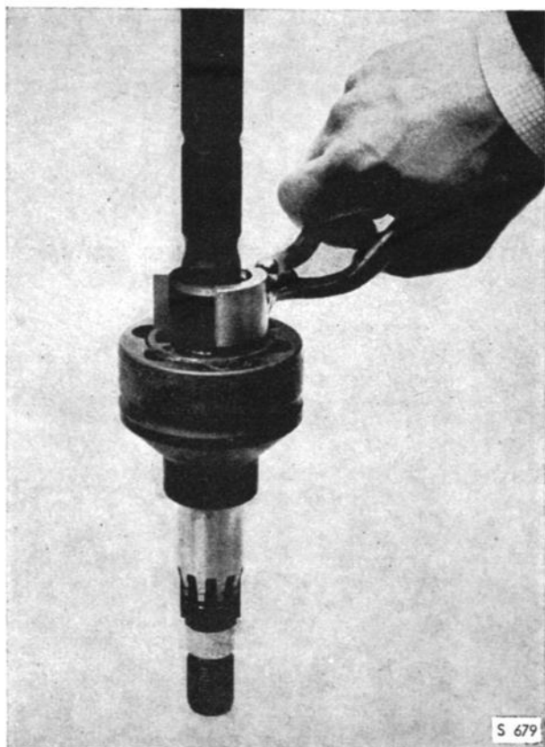
ASSEMBLY OF MIDDLE DRIVE SHAFT IN THE HUB
