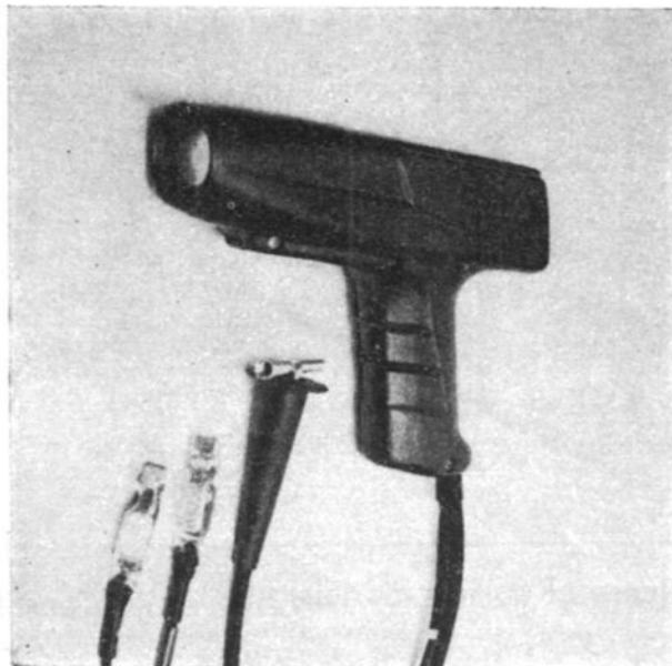
STROBOSCOPE, 12-VOLT Used for ignition adjustment. Essential.
