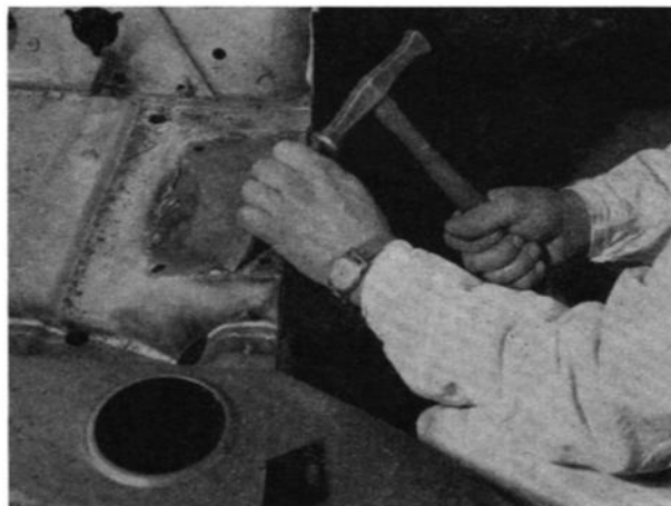
REMOVING TACK-WELDED BODY PANELS
