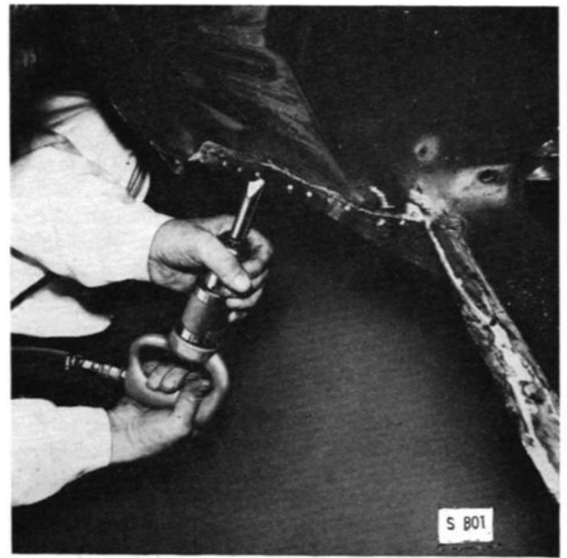
CHISELING OFF REMAINING METAL STRIPS
