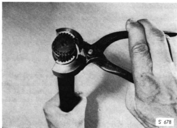
PLACING THE LOCK RING IN TOOL 784161
