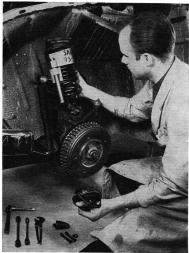
REMOVAL OF FRONT COIL SPRING WITH TOOL NO. 784082
