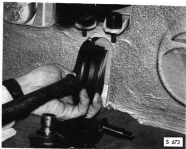
REMOVAL AND INSTALLATION OF INNER DRIVE SHAFT
