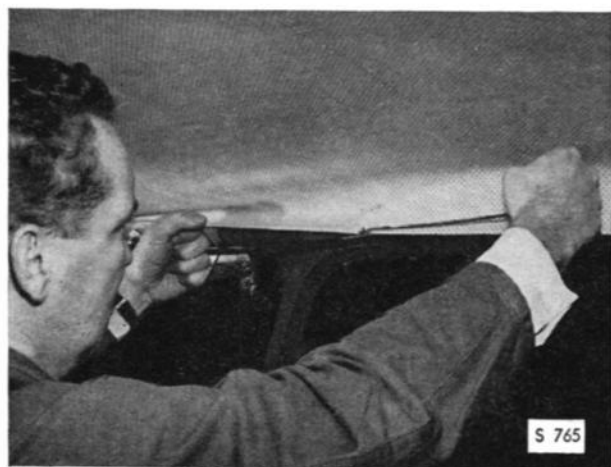
STRETCHING THE WIRE SPIRALS, SAAB 95
