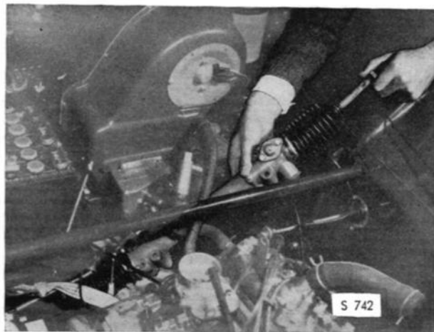
REMOVAL OF STEERING GEAR
