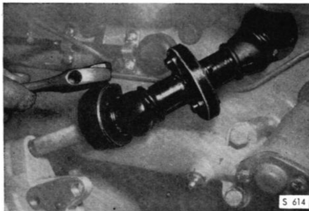
REMOVAL OF GEAR-SHIFT SHAFT, TOOL 784083
