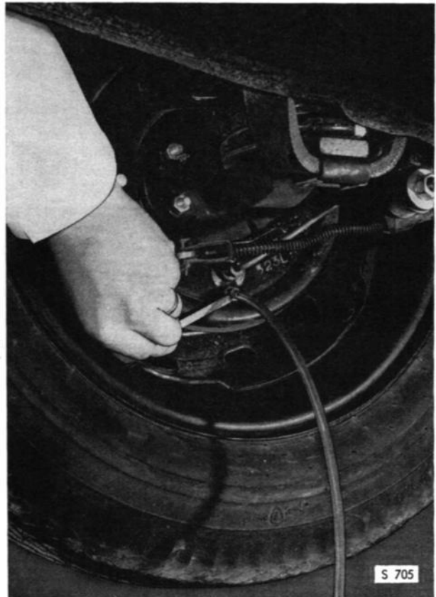
LOCATION OF BLEEDING NIPPLES, REAR END, SAAB 95, 96 AND SAAB SPORT
