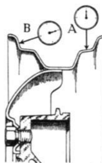
MEASURING OUT-OF-ROUND AND RUN-OUT
