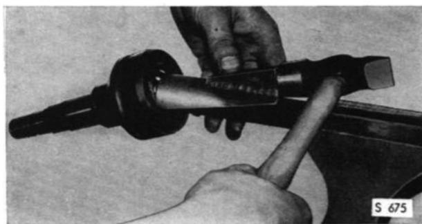
REMOVAL OF HUB WITH ARBOR 784165
