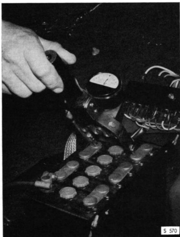
CHECKING THE BATTERY WITH A CELL TESTER
