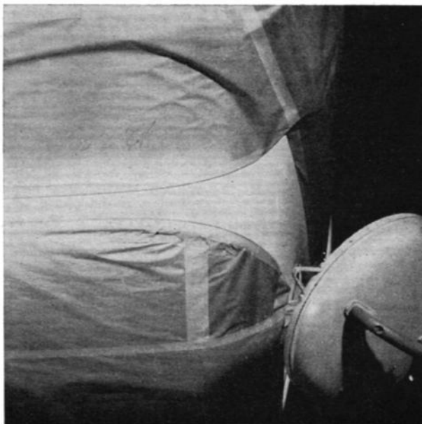
USE OF RADIATION LAMP TO DRY REFINISHED PART
