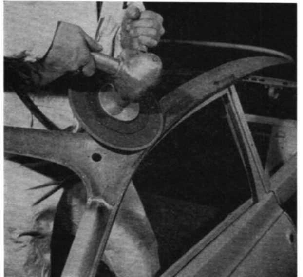
REMOVING WELD REMAINS. NOTE POINT AT WHICH PILLARS ARE CUT.
