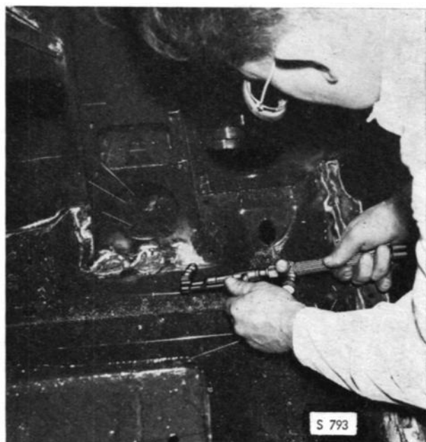
CUTTING AWAY THE WHEEL HOUSE AND CONTROL-ARM BRACKET
