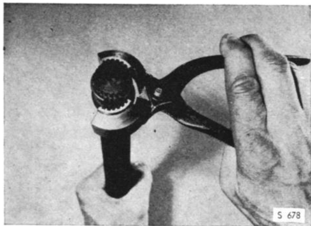
PLACING OF LOCK RING IN TOOL 784161
