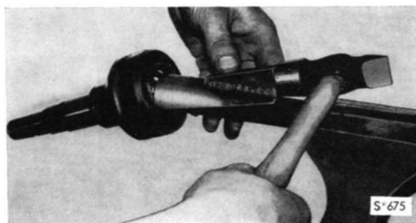
REMOVAL OF INNER DRIVE SHAFT FROM OUTER UNIVERSAL JOINT WITH TOOL 784165
