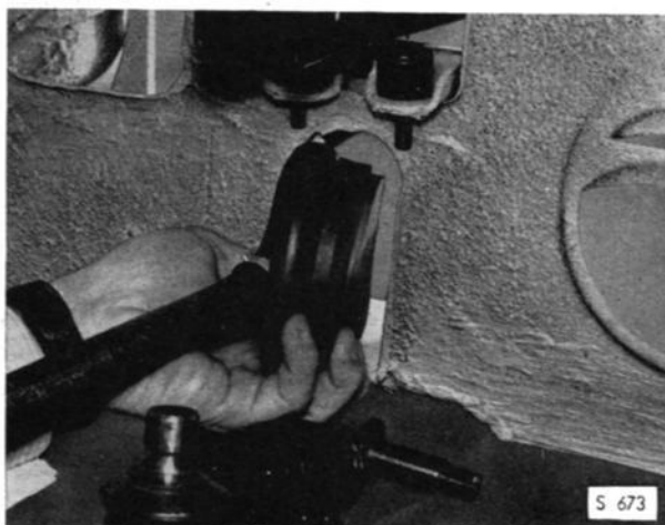
REMOVAL OF MIDDLE DRIVE SHAFT
