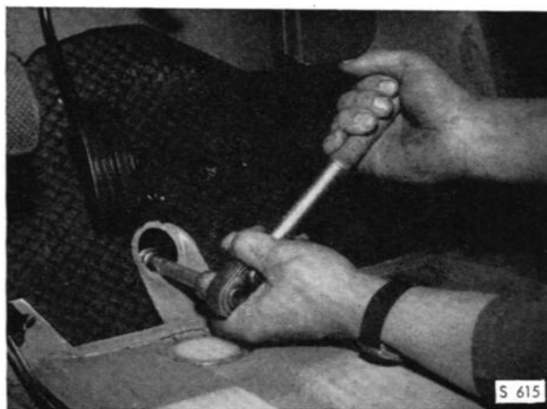
REMOVAL OF THE REAR ENGINE BRACKET CENTER SCREW
