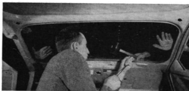
FITTING WINDSHIELD STRIP WITH LEATHER THONG
