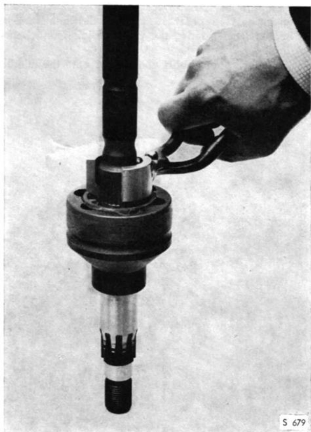
INSTALLATION OF INNER DRIVE SHAFT
